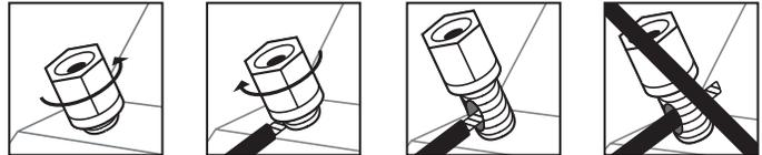
To connect wire to the binding post [see figure above], unscrew the knurled nut and insert the bare wire into the hole near the base of the binding post. Do not insert the insulated part of the wire into the hole as this will not give you a good connection. Twist the nut back down the binding post until it firmly meets the wire. Do not over tighten.
