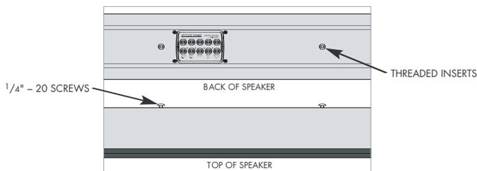
1. Two 1/4"-20 screws have been factory installed on the back of the speaker. Gently hand-turn the screws to make sure they are in as far as they can go. Do not force them beyond the “stop” point. The screws cannot screw all the way into the speaker and should protrude as shown in the illustration.
