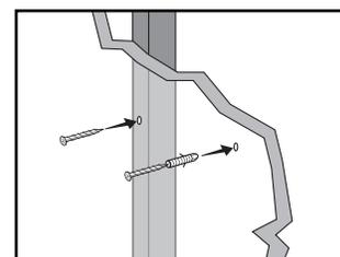
10. For masonry walls, use a masonry drill bit to pre-drill holes, and use masonry anchors and screws (not included).
