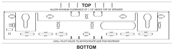
5. Use a bubble level to make sure the template is level. If the TV is wall mounted and not level, the speaker will look better if it is off-level in exactly the same way as the TV.
