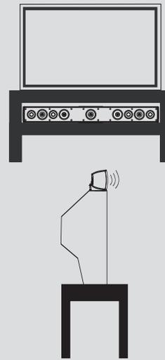
If placed on a shelf under a TV, adjust the leveling feet (screwed all the way in) to aim the speaker up towards the listeners.
