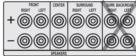
If you have a 6.1 or 7.1 channel receiver, connect the SSA's surround channel inputs to the "Surround" outputs of your receiver, not the "Rear" or "Surround Back" outputs.
